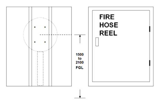
Please note: back fixing panel for reel mount bracket is extra. nominate the brand of reel for correct fixing.
